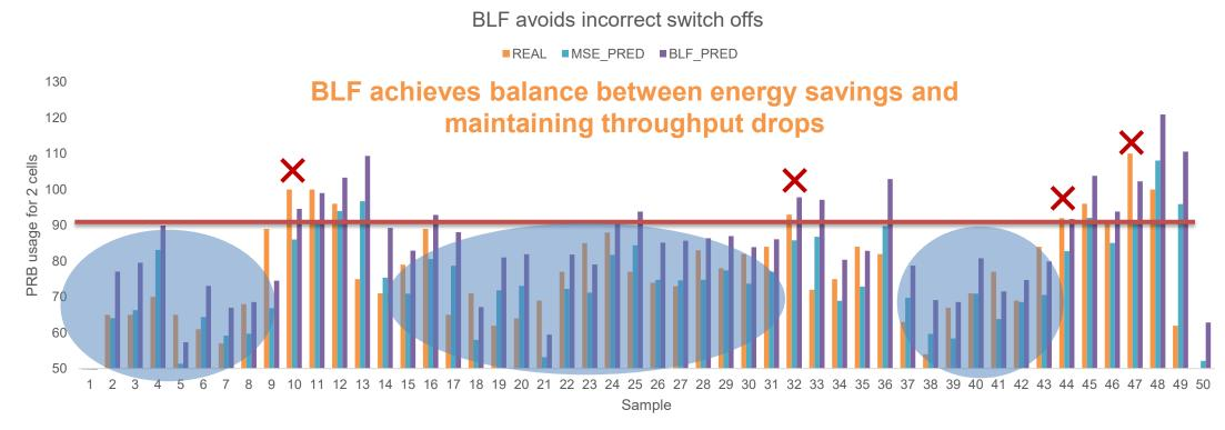
BLF backed predictor is able to **reduce the incorrect switch off instances by >2x** w.r.t. standard loss functions. (36 instances of wrong switch offs vs 15 instances, if BLF is used across ~400 samples. **Threshold chosen is 90**)
