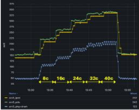
Fig. 4. Characterization and comparison of power measurements from PDU (green), IPMI (yellow), and Kepler (kepler_node) utility. Server load request increases from 8CPUs to 40CPUs, in steps of 8CPUs every 240secs.
