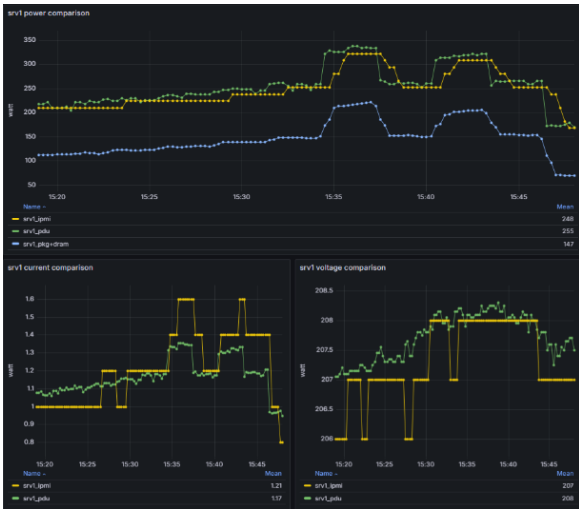
Fig. 5. Top: Power measurements from PDU (green), IPMI (yellow), and Kepler for small and large increases of CPU load. Bottom left/right: Current and voltage from PDU and IPMI, showing the relatively coarse granularity of the IPMI metrics.
